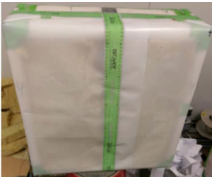
Overlappend dampscherm met tape
